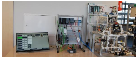
Fig. 1. Laboratory station for cyberattack simulation
